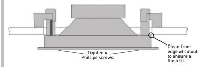
Insert the speaker into the hole and tighten the four toggle screws. As you start to turn each screw the toggle clamps will rotate outward to engage the ceiling or wall material as shown. CAUTION: DO NOT OVER-TIGHTEN THE CLAMPS. Too much torque may damage the toggle, causing the speaker not to seat securely. A snug fit is all that is necessary to assure proper performance.
